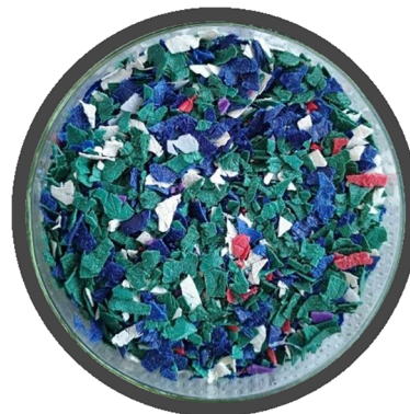
Figure 1. High-density polyethylene (HDPE) particulates.
